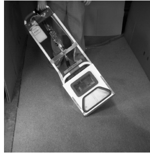
Figure 21: Tilt machine to right to manually activate discharge pump
