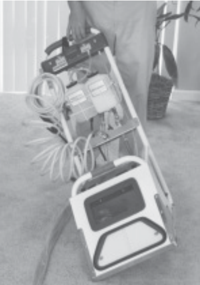
Figure 19: Manually Activating Discharge Pump By Tilting Machine to the Right
