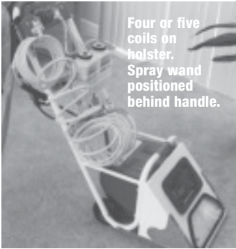
Figure 12: Properly Hung Prespray Hose
