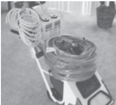
Figure 21: Hoses Secured With Bungee Straps
